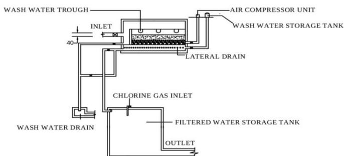
Fig 4: Typical Section of Rapid Gravity Filter
