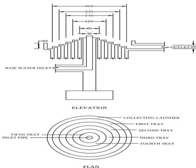
Fig 2: The elevation and plan of cascade aerator.
