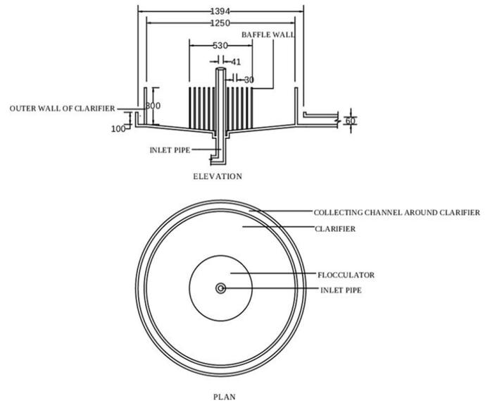
Fig 3: Elevation and Plan of Clariflocculator
